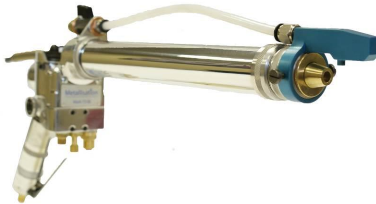
Extension unit shown fitted to the MK73 flame spray pistol
